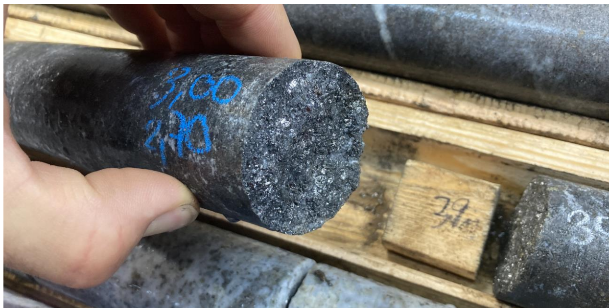
Figure 12-1 Part of a Sample in Hole AS23-14 that Grade 14.3 %Cg Over 1.4 m
