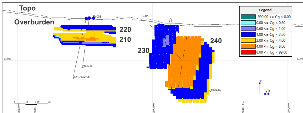
Figure 14-11 Section 200 – Showing Estimated Block Model
