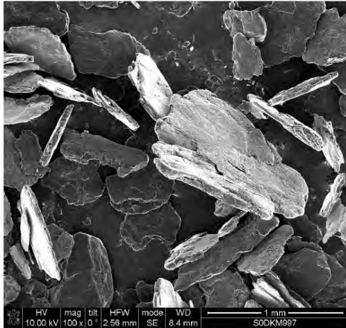
(100 X magnification) Large, platy graphite crystals, up to 1mm size, or more (+16 mesh).
